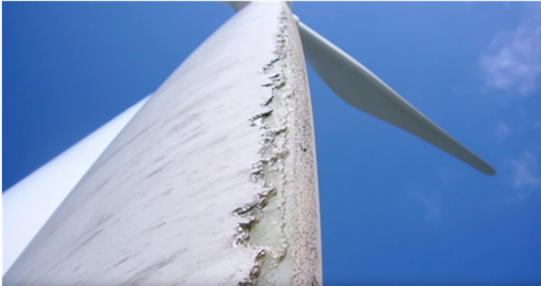
Figure 6.1 Leading edge erosion of a wind-turbine rotor blade (@MarkELacey).
